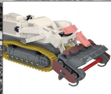
Access to key locations for the front tool maintenance.
