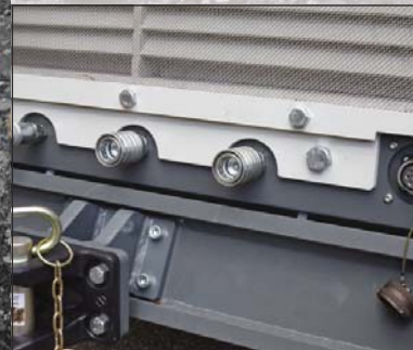
Rear : hydraulic quick coupling and electrical connection (CAN bus and power supply).
