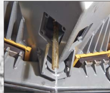
Access for hydraulic and fuel tanks drainage
