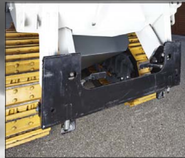
Front: Caterpillar mechanical quick coupler. Potential use of all the compatible Caterpillar tools.
