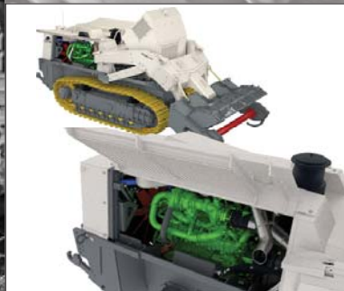
Automatic (or manual) access for Diesel engine servicing (Diesel filters, gauge, oil, intake filters, ...)
