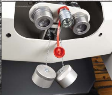
Front : hydraulic quick coupling (250 litres/minute at 400 bar) and electrical connection (CAN bus and power supply).
