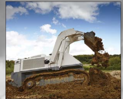
Front : arms lifting capacity : 2 tons at four meters height.
