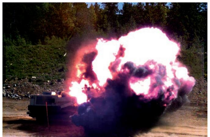
Detonation of the equivalent of 8kg of TNT.
