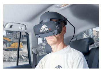
Via a high speed radio link with no perceptible latency, the operator finds himself immersed in the control of his vehicle thanks to a Virtual Reality (VR) headset.
