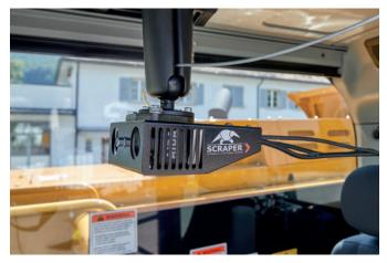
The stereoscopic camera can be installed in just a few seconds in the space usually occupied by the operator's head.
