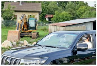
The remote control station can be adapted to suit different surroundings such as the back seat of a car or a permanent container for longer working periods. A quiet generator permits independent use.
