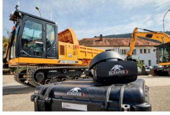
A vehicle equipped with SCRAPER can always be controlled directly from the cab when there is no risk of danger. The SCRAPER system contained in two suitcases can be deployed rapidly at any time, as required.
