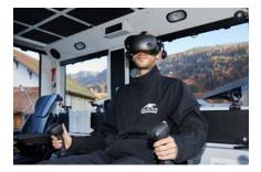
In addition to the screens, a stereoscopic view through a VR headset allows precision operations to be performed as if you were in the machine.
