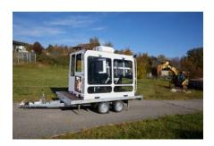
Optional: the cabin can be supplied on a road trailer fitted with stabilisers for levelling.
