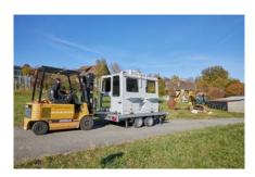
The cabin can be moved using a forklift truck. Lifting points also allow the cabin to be moved by crane.
