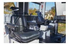
One operating station equipped with joysticks and pedals.
